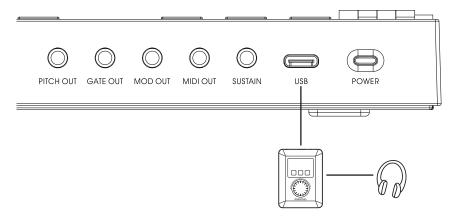
Use with **miDiPLUS** miniEngine series sound engine: Connect Vboard 25 to the USB Host of miniEngine using the included USB cable, hold down the Power button to turn on the power. connect your speaker or headphone to miniEngine and turn on the miniEngine.
