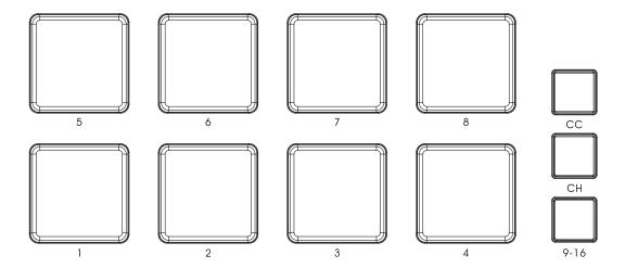
Vboard 25 features 8 velocity and pressure sensitive pad with backlit, they has 3 working modes included MIDI Note, MIDI CC and MIDI Channel.
