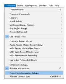
2. Select the **Machine Control** and enable MMC Slave Active, set the **MIDI Input** and **MIDI Output** as **Vboard 25**, then set the **MMC Device ID** as 116
