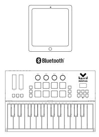
Use with iOS device: Hold down the power button to turn on the power, and turn on Bluetooth on your iOS device, lanuch the APP which support Bluetooth MIDI and connect Vboard 25 in setup menu. Please refer to 5. Bluetooth MIDI Connect(iOS).
