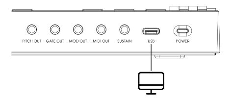
Use with computer: Connect Vboard 25 to your computer using the included USB cable. Hold down the Power button to turn on the power. Vboard 25 is a class-compliant USB device, so its drivers are automatically installed when connecting to a computer.
