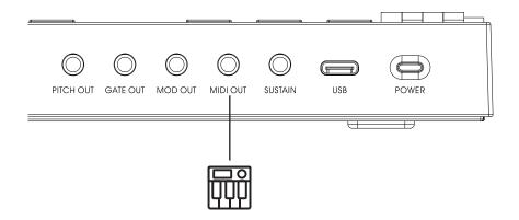
Use with external MIDI device: Connect to a USB 5V power adapter using the included USB cable, connect the MIDI OUT of Vboard 25 to MIDI IN of external MIDI device with a 5 pin MIDI cable.
