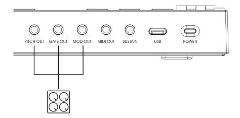
Use with analog synthesizer: Connect the Vboard 25's pitch out, gate out and mod out to the analog synthesizer's CV inputs using 1/8" TS cables, Vboard 25 can be power by the build-in battery.
